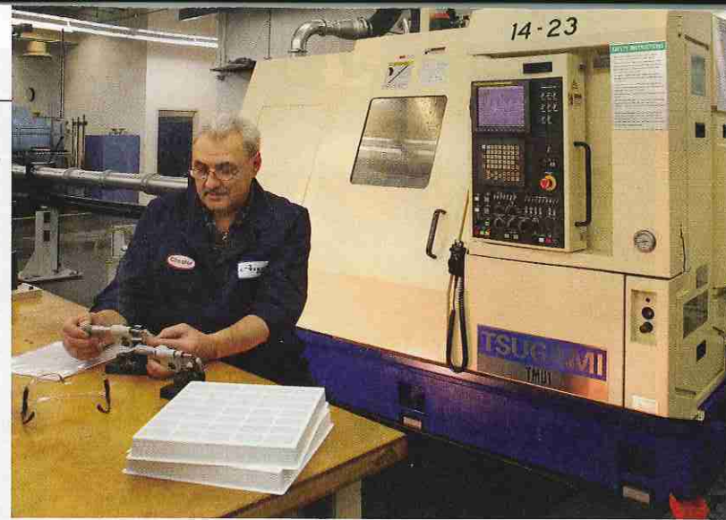
▲ Chester Pogorzelski monitors part features during runs on this Swiss-type machine. Quality control is more an insurance policy now at Tier One. Rarely do they discover rejects. Scrap is negligible.
