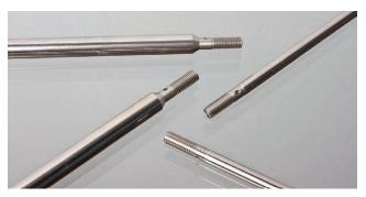
▲ Here is a sample of some of the parts that run across the Swiss machines. Prior to installing the Swiss machines, these parts were processed with several handlings. Now they come off the machine tool complete.
