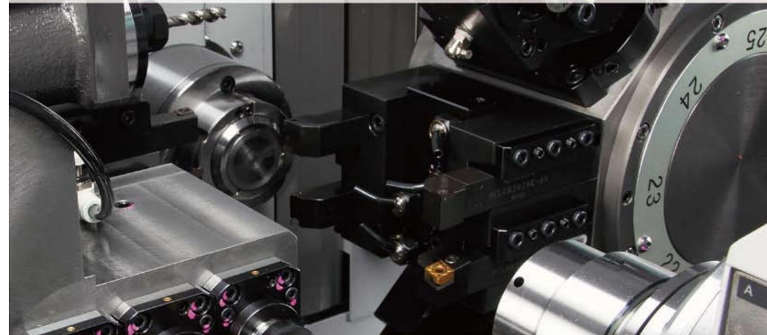
A sliding headstock type automatic lathe that encompasses the entire process
